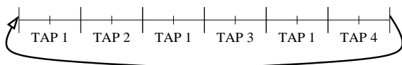
Figure 5: A TAP schedule loop in which TAP 1 must be run more often than the others.
